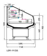
BCA – low glass or front glass riser | single, bent | fixed CSS – cover | single, straight | sliding (sideways)
