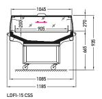
**BCA** – low glass or front glass riser | single, bent | fixed **CSS** – cover | single, straight | sliding (sideways)
