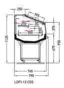
**BCA** – low glass or front glass riser | single, bent | fixed **CSS** – cover | single, straight | sliding (sideways)
